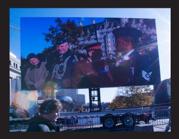
Impact's DOMINATOR® HD large screen trailer mounted LED display is perfect for any outdoor event. The screen can be set up in as little as 60 minutes and is ideal for outdoor applications that require a high quality screen with limited set up time. The DOMINATOR® HD package contains a full on-board control room with switching capability that supports most video playback formats. Additional capabilities include multi-camera packages, real time data & scoring feeds, as well as graphics production.
